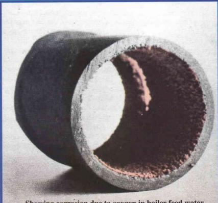
Showing corrosion due to oxygen in boiler feed water
